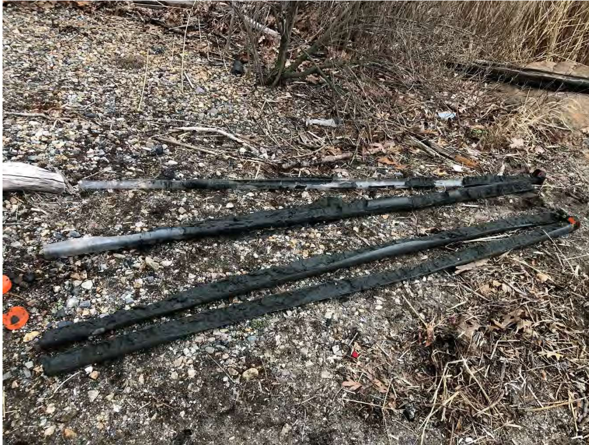
Photo 1: View of Chem-6. Top run from left to right from 0 to 10.2 ft, bottom run from left to right 10.2 ft to 21 ft.
