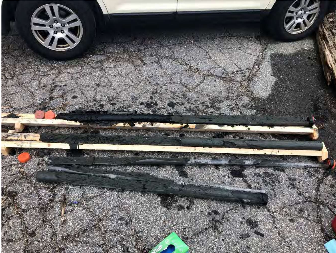
Photo 1: View of Chem-2. Top run from left to right from 0 to 7.2 ft, middle run from left to right 7.2 to 14.8 ft, bottom run from left to right 14.8 to 18.6 ft.
